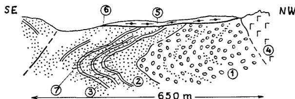
Fig. 4. - Detail of a section along the left slope of Khibelen river, showing a thrust surface cutting and underlying fold structure in the middle Proterozoic. 1 : conglomerate; 2 : inequigranular sandstones; 3 : siltstones; 4 : gabbro; 5 : early Proterozoic mylonitic plagiogranites; 6 : fault surface; 7 : cleavage.
